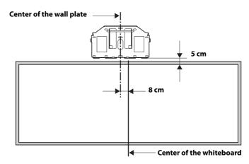
2) Position the wall plate over the marks you made in step 1, and then mark the points where the wall plate will be secured as shown in the following illustration.
